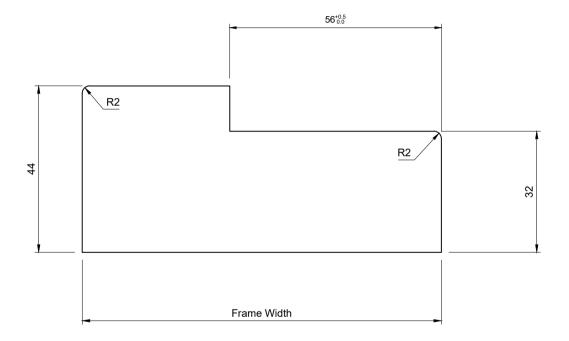
Description: Machining Profile Timber System 2 - 44/32 Profile - NFR - 54mm Door - Non-Acoustic - Non Q2F
